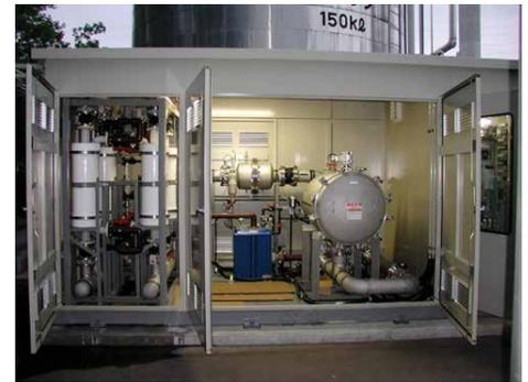
automation and a feed back signal, the soft water is controlled to a pH of 5.0 with sulfuric acid. Caustic soda is added daily to inhibit bacteria growth. Very minimal chemical usage is required to control the pH.
