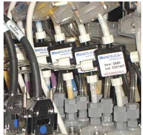
3M™ Liqui-Cel™ SP-0.5x1 Series Membrane Contactors installed on a wide format ink jet printer
