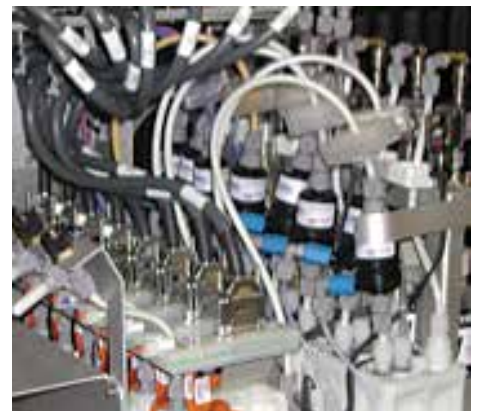
3M™ Liqui-Cel™ SP-1x3 Series Membrane Contactors installed on a wide format ink jet printer.
