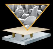
Conventional ceramic abrasive grain tends to "plow" through the metal, causing heat to build up in the workpiece and the abrasive — resulting in a slower cut and shorter disc life.
