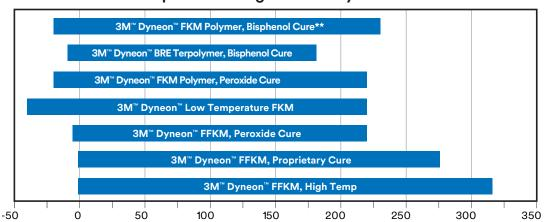
Temperature range in °C; test results based on retention of physical properties
