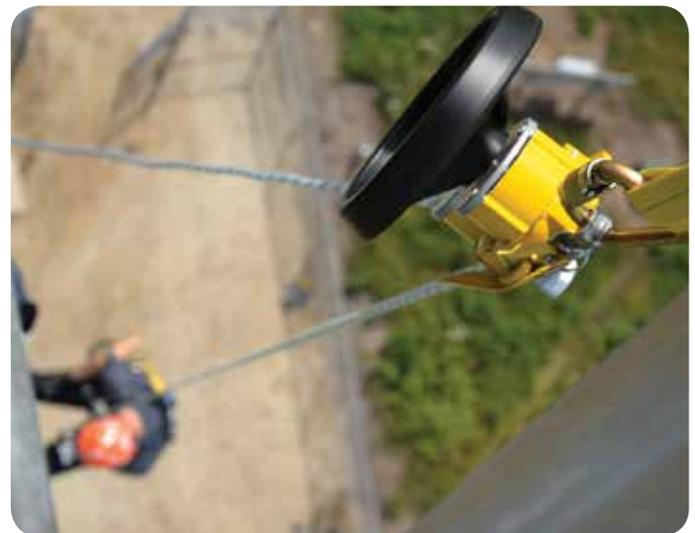
device to be removed, and then lowered to the ground safely. With a drill attached, the R550 can also provide lifting capabilities which is essential in confined space rescues.
