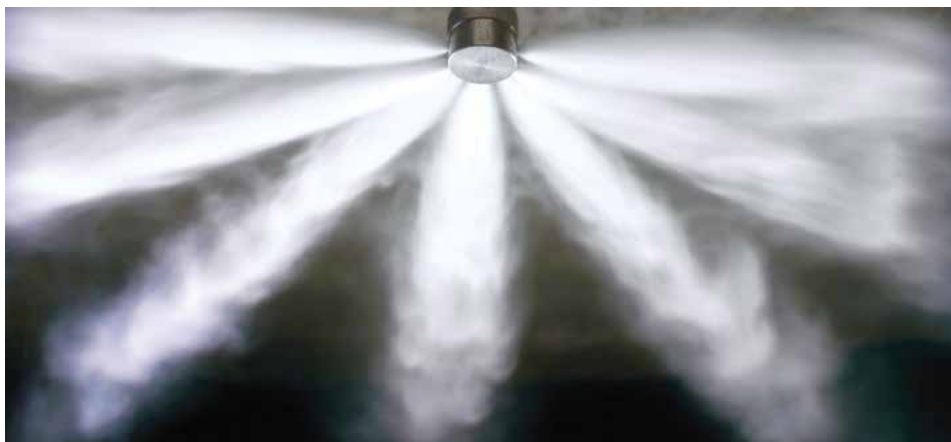
3M's Novec 1230 fluid for fire protection
