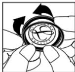
Insert the flexible edge of the diaphragm into the groove of the rim. This is best accomplished by starting with the rim positioned above the legible side of the diaphragm.
