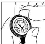
Visually inspect the edge where the diaphragm engages the rim for uniform containment. Minor adjustments may be made by slightly pulling and rolling the rim away from the diaphragm, allowing the diaphragm to slip into position.
