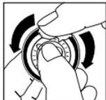
Using your fingertip, apply a small amount of talcum powder to the inside surface of the flexible edge of the diaphragm. This will facilitate assembly and maintain smooth and quiet low/high frequency alternation. Snap the diaphragm with your fingers to remove excess talc.
