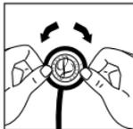
With the diaphragm side up, grasp the rim with the thumbs and index fingers of both hands and roll the rim off the edge of the chestpiece. Remove the diaphragm from the rim and clean the parts in soapy water or wipe with alcohol. Chestpiece surfaces can be wiped with alcohol or soapy water. Dry all parts and surfaces thoroughly before reassembly.
