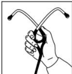
To increase spring tension, grasp the headset with one hand where the eartubes enter the tubing and squeeze until the tubing on one eartube touches the other. Repeat as necessary.
