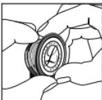
To attach the rim/diaphragm assembly to the chestpiece, engage the groove of the rim (with the diaphragm attached) around the chestpiece at one point and hold it in place with your thumbs.
