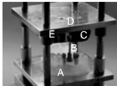
Figure 33. Model (A) in the impression rig. The suitable rim-lock tray (C) is mounted to the base plate (E) and can be lowered to the correct position. Post (B) will then jutt out of hole (D).
