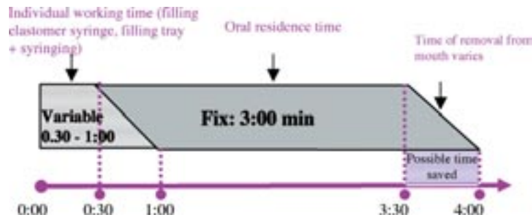
Figure 3. Setting times for the fast setting Soft Quick Step polyether product line
