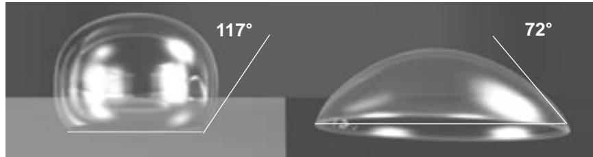
Figure 8. Water droplet on A-type silicone (left) and Impregum Penta Soft (right). In contrast with A-type silicones, a smaller contact angle will form immediately after the first contact of a water droplet with Impregum Penta Soft due to its intrinsic hydrophilic nature.
