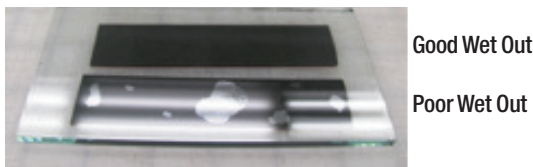
Figure 9. A piece of glass showing good wet out of the tape vs poor wet out.
