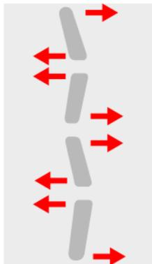
Special temple design with multiple struts provides constant pressure equalisation.
