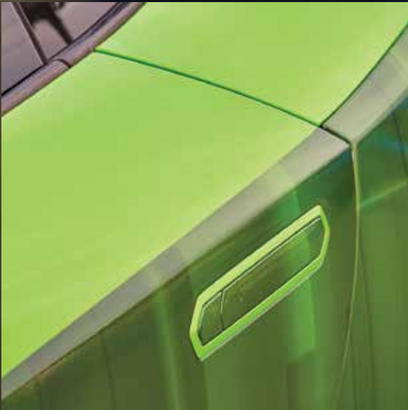
▲ Green vehicle colour shows through film and is part of the design.
