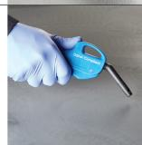
Blow off the surface with clean dry air and then use a VOC compliant surface cleaner to remove any remaining residue.
