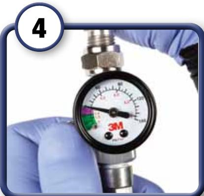
4 Set air pressure at 25 psi for 1<sup>st</sup> stage (only air flowing)
