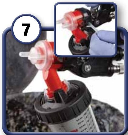
When you are finished using the system, pull the trigger back to release fluid back into cup, remove the air line, and the 3M™ PPS™ Cup.
