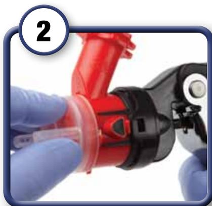
Attach an atomizing head to the gun - pull trigger back and hold, making sure the release buttons are aligned with latch openings - listen for a double click to ensure that it is fully engaged.
