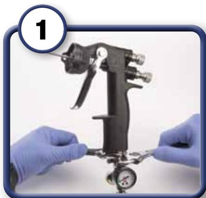
Hand tighten or use two wrenches to connect the air flow control valve.
