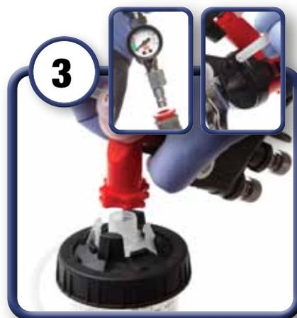
Attach 3M™ PPS™ cup filled with coating and attach compressed air hose.
