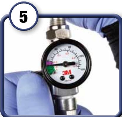
5 Set air pressure at 15 psi for 2<sup>nd</sup> stage (air and fluid flowing)
