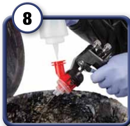
Flush out atomizing head with appropriate solvent until the atomizing head is clear of coating.
