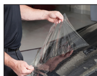
Paint Protection Film Virtually invisible film to protect vulnerable vehicle surfaces
