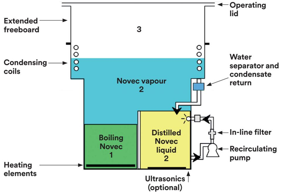
3M™ Novec™ Engineered Fluids are also suitable for use in a co-solvent process.
