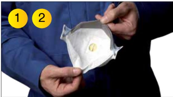
1. With the reverse side up and using the tab, separate the top and bottom panels of the respirator to form a cup shape. Bend slightly at the centre of the noseclip.
