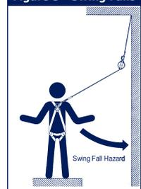
**Figure 4 - Inappropriate Connections**
