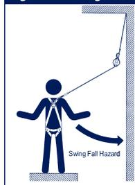
**Figure 4 - Inappropriate Connections**
