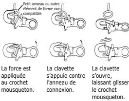
**Figure 5 - Connexions inappropriées**
