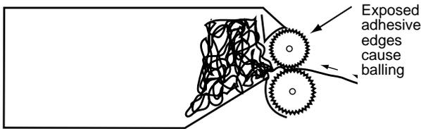
**Note:** This figure shows the balling up of the cover tape that restricts forward movement and causes jamming of the feeder.
