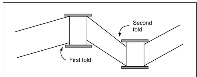
**Note:** The initial solution was successful in folding the adhesive edges and reducing adhesive residue and jamming, but it proved difficult to thread in the startup of a new reel.
