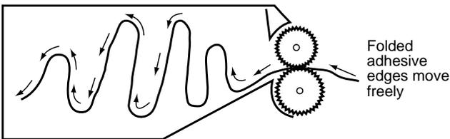
**Note:** This figure shows cover tape with the adhesive edges folded over and a normal flow through the collection bin.
