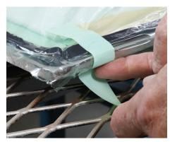
Works outside the bagging area to securely hold/position bagging materials and thermal couple wires while providing clean removal from tooling post cure.
