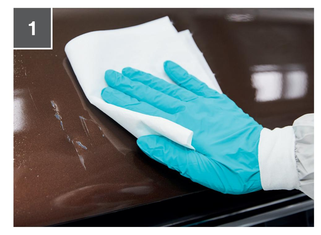
Inspect the damaged area and degrease in accordance with paint company recommendations.
