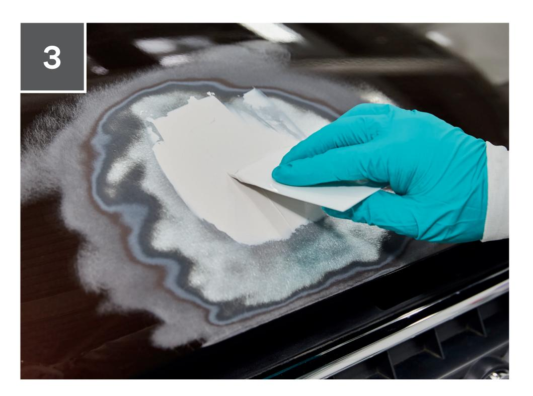
Mix and apply body filler to damaged area, avoiding surrounding paintwork. Reshape panel as required.
