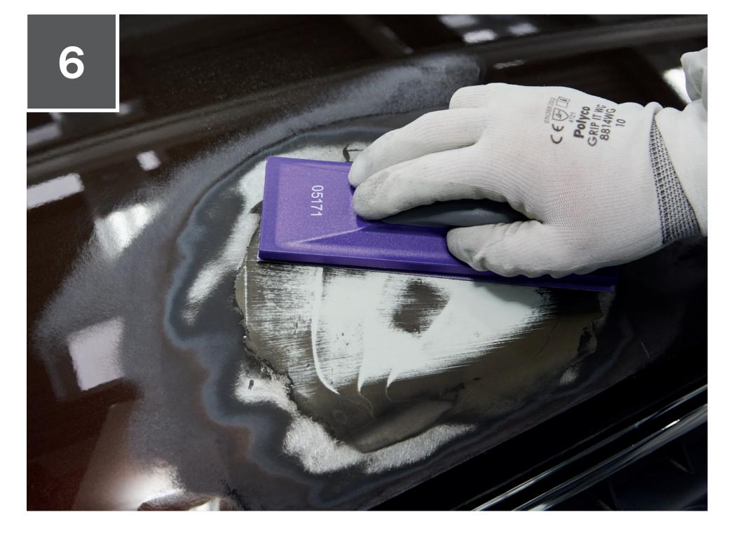
Apply 3M Dry Guide Coat and hand sand the filler or glaze to the required shape and finish using using a P180 abrasive.
