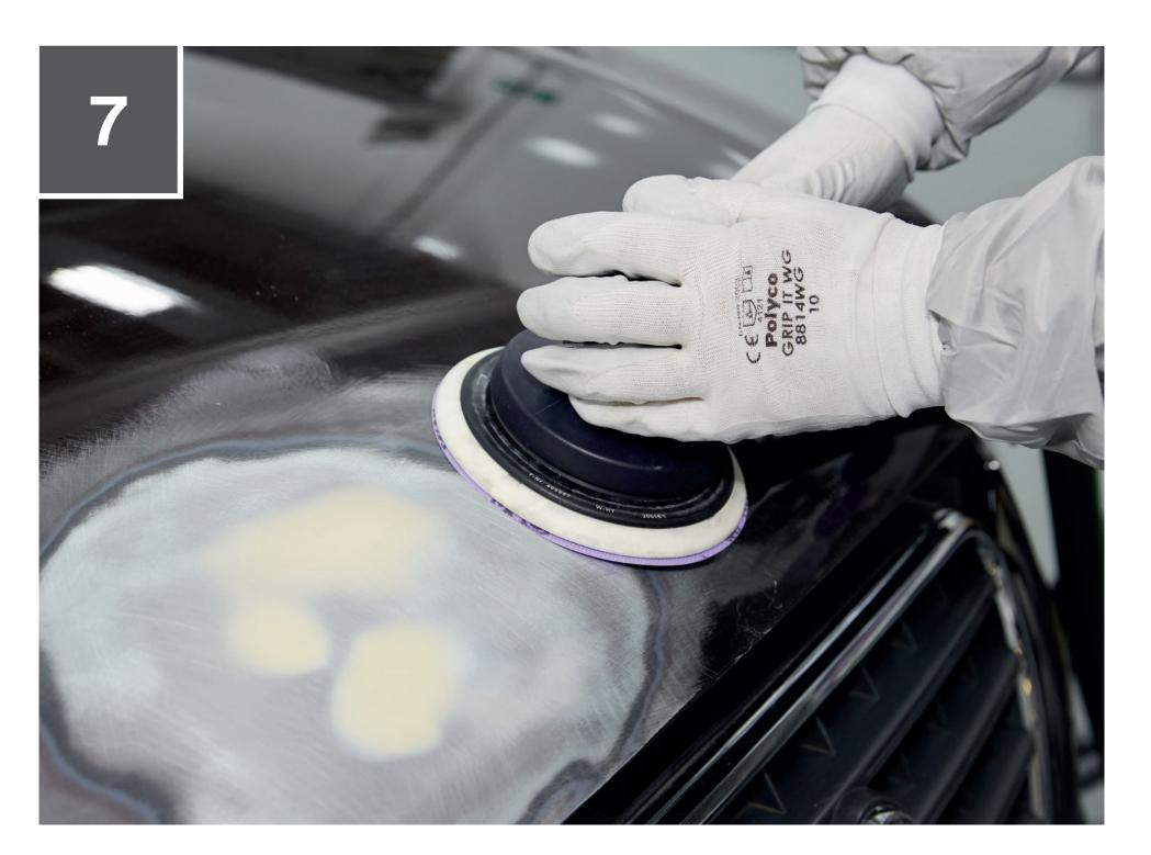
Feather around the repair area ensuring that any deep scratches are removed using a finer grade abrasive.
