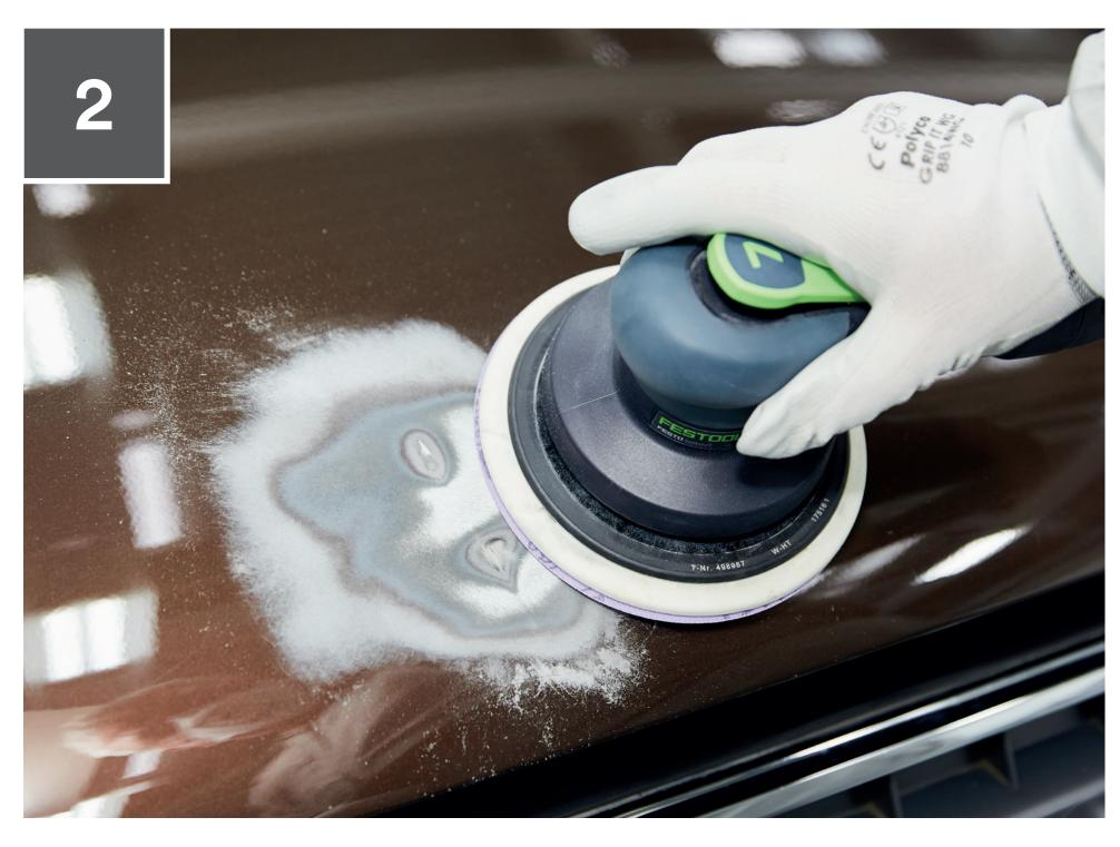
Remove paint from the damaged area using a dual action sander combined with the relevant 3M abrasive, ranging from P80 to P120 grade.
