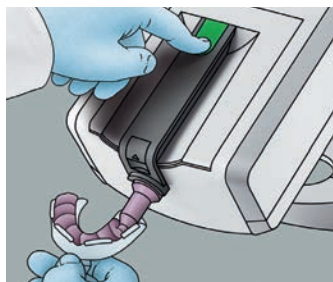
7. Press the green start button to fill the impression tray or elastomer syringe.
