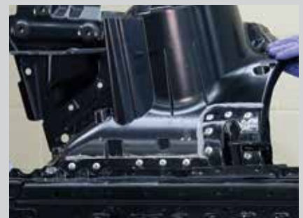
Adhesive bead starts silver in color and changes to purple once curing has begun
