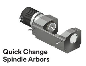
Quick change spindle arbors are special outboard dressers designed to address larger grinding applications with frequent change over or high part mix. These dressers feature a retractable spindle assembly allowing efficient arbor removal.
