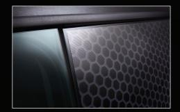
▲ Create a uniform relief cut between window graphic and rubber molding.
