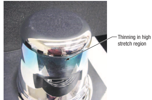
Figure 7. Effect of thinning in high aspect ratio part
