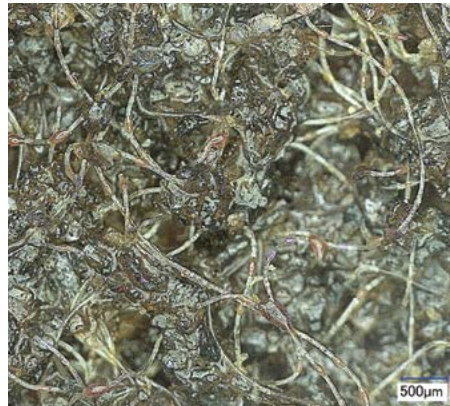
Scotch-Brite Weave, Pictured at 500 µm
