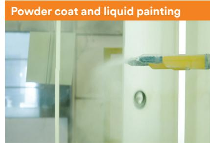
3M™ VHB™ Tape GPH's high temperature resistance allows it to be bonded prior to powder coat or liquid painting processes. This reduces the number of "touches," leading to a more streamlined manufacturing process.
