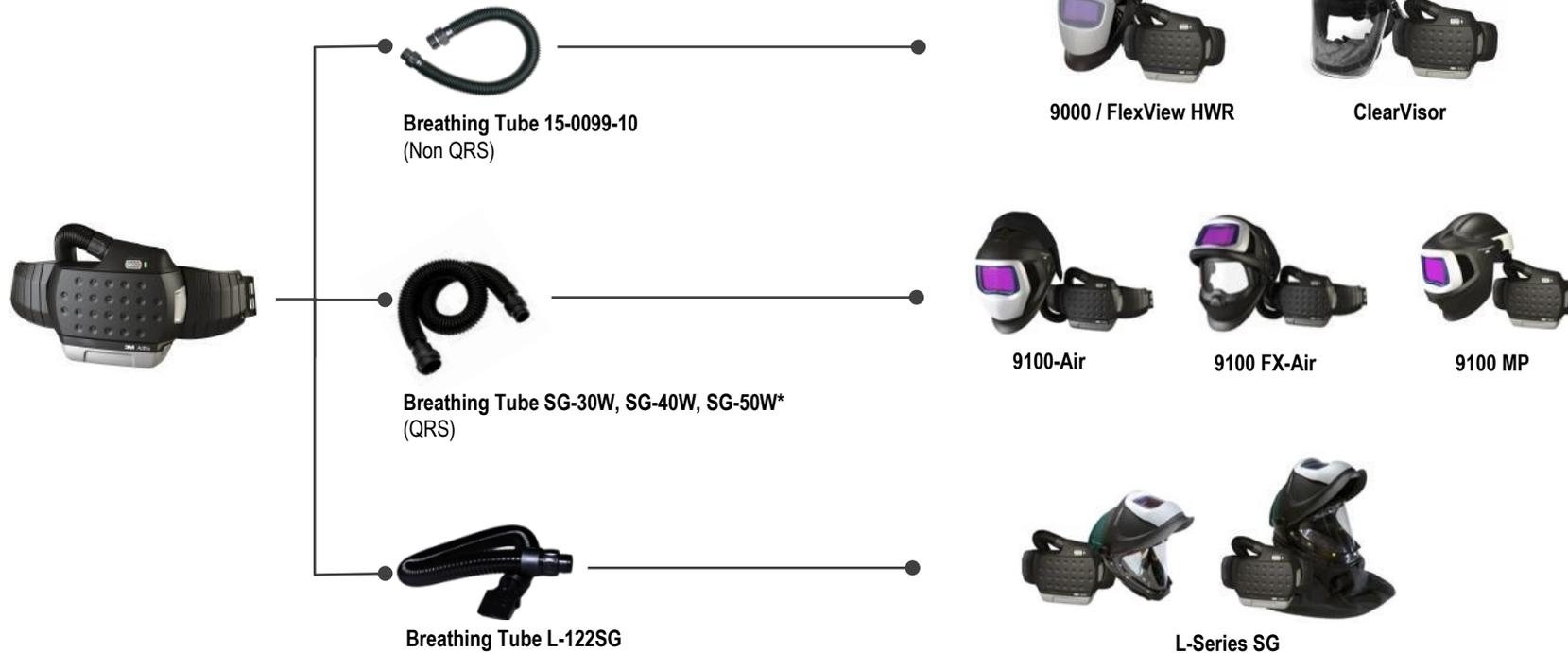
\* When using the Adflo PAPR with HE filter + OV/AG cartridge together with Speedglas welding helmet 9100-Air or 9100 MP, the SG-50W breathing tube must be used to be compliant as a NIOSH-approved system.
