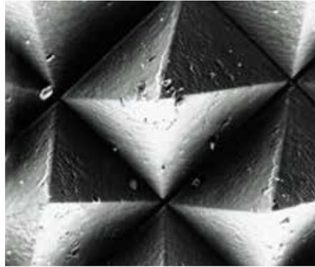
Three-dimensional structures uniformly distributed over the entire surface of 3M™ Trizact™ Abrasives (shown left) ensure consistent performance and eliminate belt-to-belt variation. Conventional abrasives, which feature randomly arranged minerals, wear and finish unevenly.
