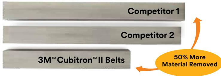
This photo shows three identical 304 stainless steel bars after nine grinding cycles of ten seconds per cycle using equal pressure. In that time, the Cubitron II belt removed more than 50% more metal than the so-called “next-generation” ceramic grain abrasive.
