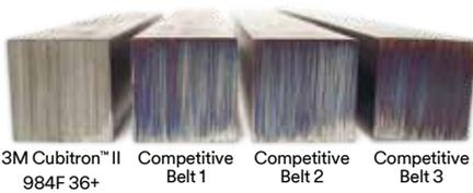
This photo shows four identical 304 stainless steel bars after nine grinding cycles of ten seconds each. While the three bars that were ground using conventional ceramic abrasive belts show varying degrees of oxidation, the bar ground with a Cubitron II belt is free of burnishing.
