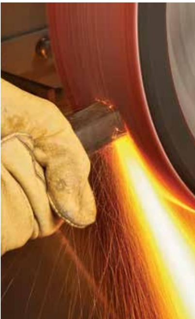
As shown by the sparks in this photo, Cubitron II abrasives divert heat to the swarf, keeping both the workpiece and the belt cooler.
