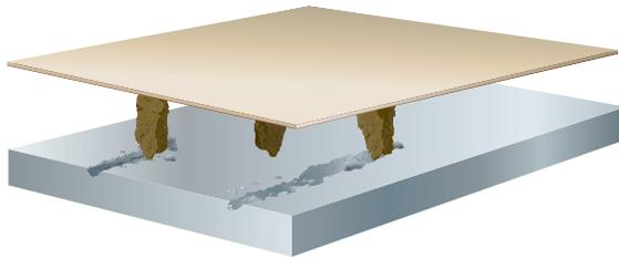
Conventional ceramic abrasive grain is irregular and blocky in shape. Instead of a clean, machining action, the grain tends to “plow” through the metal, causing heat to build up in the workpiece and the abrasive – resulting in a slower cut, shorter belt life and undesirable effects, such as burnishing.
