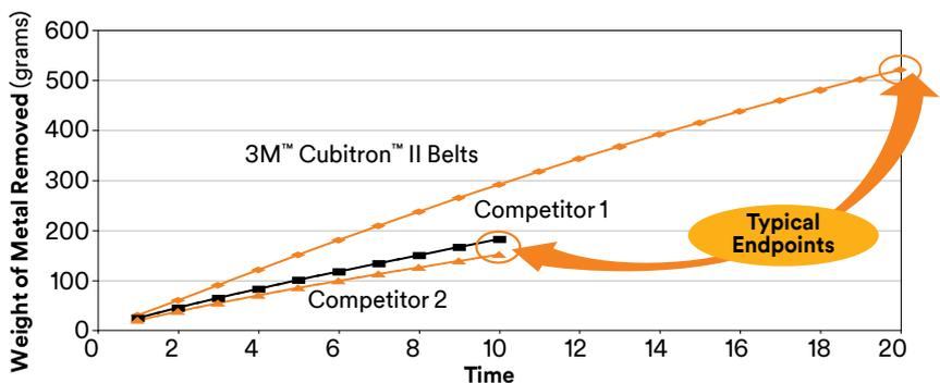
3M surveys indicate that most operators stop using a belt when performance drops to 2/3 of its initial cut rate. As this graph shows, Cubitron II belts take twice as long to reach that end point as conventional ceramic abrasive belts. In addition, Cubitron II belts cut faster throughout their entire life. Bottom line? Not only is more work done per unit of time, but also much more total work per belt.
