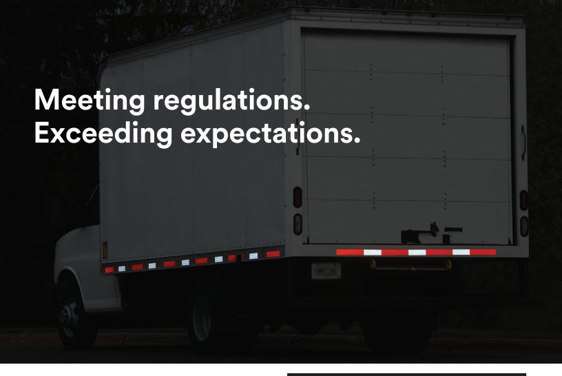
3M<sup>™</sup> Flexible Conspicuity Tape Series 913 offer color properties and retroreflectivity values that meet the FMVSS 108 regulation. Plus, it gives you the flexibility you need to give your vehicles and equipment outstanding visibility.
