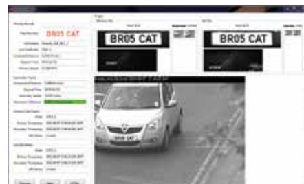
Violation details showing front plate
