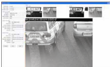
Violation details showing two plates
