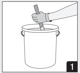
Remove lid from pail. If necessary, stir 3M<sup>™</sup> FireDam<sup>™</sup> 2000 Coating. Dilute with water to adjust viscosity for spray applications.
