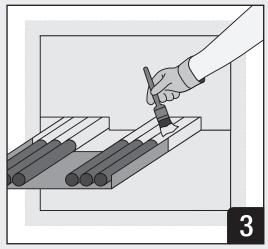
\*Allow 2–8 hours of drying time depending on thickness of coating, humidity and temperature.
