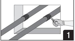
Where applicable, install appropriate firestop around through-penetrants as per system specifications (e.g., Ultra GS around elastomeric insulation, sealant around cables). Frame the opening if necessary.
