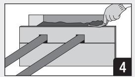
Mortar can be built up in wall applications by pouring in stages and building up temporary shutter boards until the opening is fully filled.
