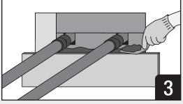
When sealant has dried install 3M<sup>™</sup> Fire Barrier Mortar in the opening. Mortar may be mixed to be stiffer (3 parts powder to 1 part water) or pourable (2 parts powder to 1 part water).
