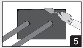
Allow mortar to cure overnight (minimum 12 hours). Remove shuttering and fill in any gaps with a stiff mortar mix.
