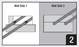
Install temporary shutter boards on the underside of a floor assembly or fully on one side and the lower half of the other side for a wall assembly, formed as closely around the penetrants as possible. Fill any gaps as needed per system specs.
