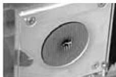
Wire-wrap sand screen. After 60 min.
