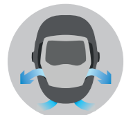
1 Exhaust vents - exhaled air is channeled out via side exhaust vents.
