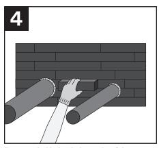
To remove the blocks/planks, gently pull them out and place on a clean surface. After penetrants are routed through or removed from the opening, replace the blocks/planks, making sure that they are firmly packed and fully filling the opening. Install foam in any voids as required.
