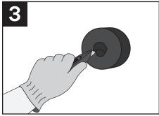
Holes may be cut/punched through plugs to route cables directly through.
