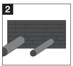
Continue to install blocks/planks until through opening is completely full and blocks/planks are firmly packed together. Block/plank can be resized in the field as needed provided the 5 in. (130mm) dimension is maintained through the opening. No compression is necessary.
