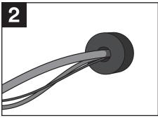
Plugs may be cut to fit around cable penetrants.
