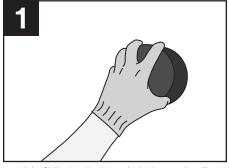
Install 3M™ Fire Barrier Plug within the opening, flush with top surface of floor or both sides of wall. To fit smaller openings, plugs may be compressed to size or a wedge may be cut from plug to reduce size.
