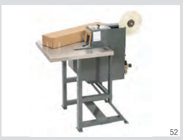
S867 3M-Matic™ L-Clip Applicator S867 is a semi-automatic unit that applies 4.5 in. L-Clips of Scotch® Filament Tapes and Scotch® Box Sealing Tapes at up to 50 clips/min.
