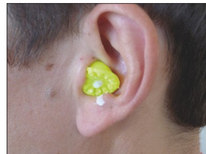
Figure 6 Earplug of Figure 5 (fitting unchanged) after the probe tube was shortened and the opening was sealed.
