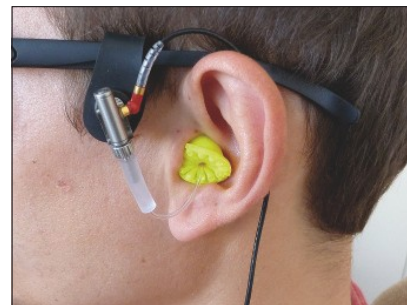
Figure 5 E-A-Rfit system with earplug with probe tube (3M E-A-RSoft FX) with connection to the measurement microphone.
