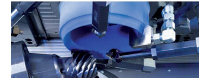
Generation grinding in bevel gear machining is a discontinuous grinding process, machining is done tooth by tooth. The generating movement of grinding wheel
