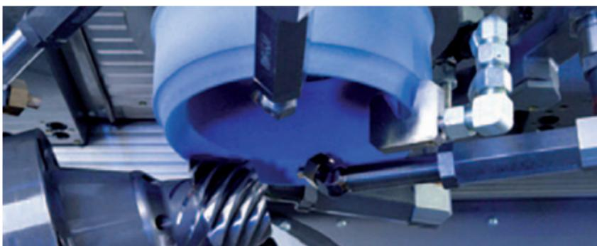
Generation grinding in bevel gear machining is a discontinuous grinding process, machining is done tooth by tooth. The generating movement of grinding wheel
