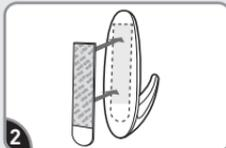
2 Remove blue liner. Press adhesive to hook.
