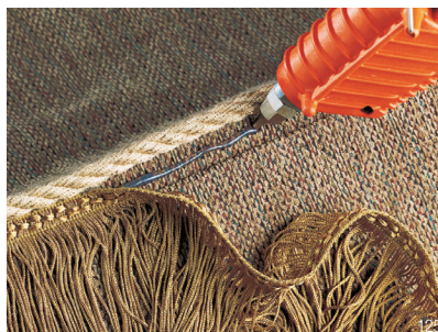
3M™ Hot Melt Applicator LT and 3M™ Hot Melt Adhesive 3792LM applied at low temperature (129°C/265°F) make quick work of welting, gimping, and bonding fabric to wood.
