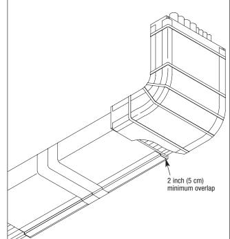
Figure 7D: Install adjacent piece of E-Mat tightly abutted to first piece. Cover the seams and exposed edges at overlap with 3M<sup>™</sup> 425 Sealing Tape.
