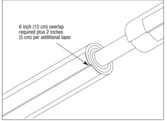
**Figure 2A:** Install 3M<sup>™</sup> Interam<sup>™</sup> Systems E-Mat layers in one continuous piece. Apply 3M<sup>™</sup> 425 Sealing Tape to seam. Install another continuously wrapped piece abutted to the piece already installed. Joint between sections may be up to 2 inches (5 cm) maximum.
