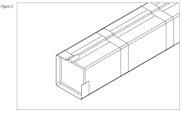
3 - Repeat these steps for all subsequent layers as per listing/design. A new stainless steel band is to be installed at the termination after the final end cap layer has been installed.
