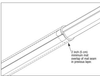
Figure 1C: Install second layer so that it overlaps the first layer seam by 2 inches (5 cm) minimum.
