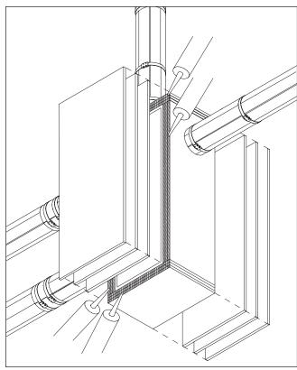
**Figure 4C:** Cut front and back mat pieces large enough to cover front and back of box and the edges of installed mat pieces. Apply  $3M^{TM}$  Fire Barrier Sealant CP 25WB+ to exposed front and back mat edges and then apply front and back mat pieces. Secure mat using  $3M^{TM}$  898 Filament Tape.
