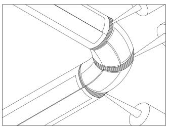
**Figure 3C:** Apply  $3M^{TM}$  Fire Barrier Sealant CP 25WB+ to fill the gaps which remain between mat sections.
