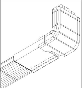
Figure 7C: Apply 3M<sup>™</sup> 425 Sealing Tape to exposed E-Mat seam.
