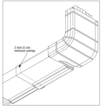
Figure 7E: Install the second layer and each additional layer with a 2 inch (5 cm) minimum overlap of the seam in the previous layer.
