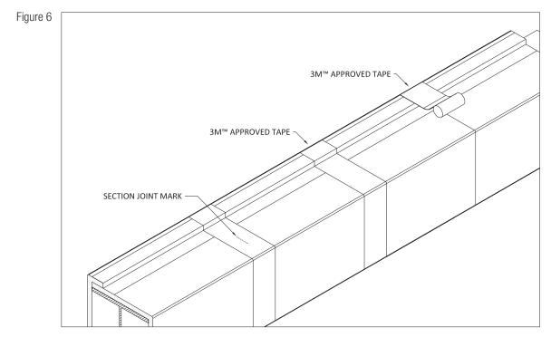
6 - If additional layers are required, measure the perimeter of the first layer and add additional length to accommodate for overlap and corner bending. Stagger the perimeter joints of the second layer by minimum of 2 inches (50 mm) away from the perimeter joints in the first layer. The reference points are used to ensure the 2 inch stagger distance. Repeat steps 1 through 5 (Figure 7)
