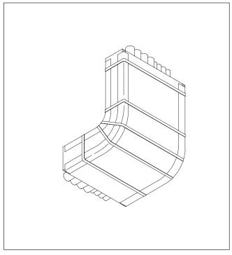
**Figure 5G:** Install steel banding around the cable tray every 12 inches (30 cm) maximum and within 2 inches (5 cm) of each cable tray elbow end. See Figures 7A to 7H for details regarding a transition of the cable tray elbows to cable tray straight sections.
