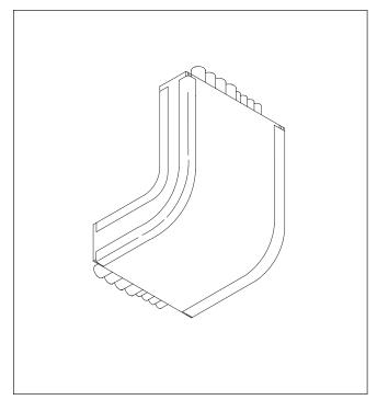
Figure 6C: Apply 3M<sup>™</sup> 425 Sealing Tape to all E-Mat seams.
