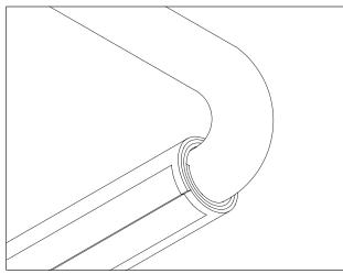
Figure 3A: Terminate straight section mat layers at beginning of conduit radius.
