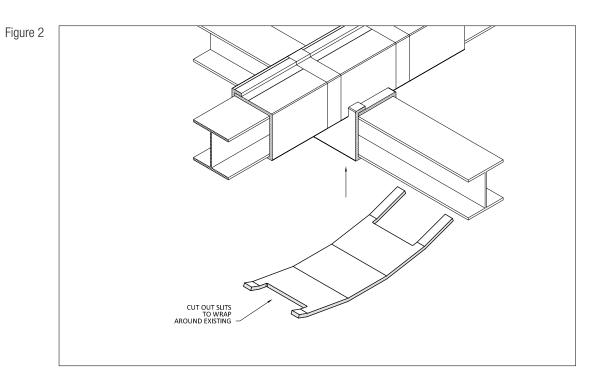
3 - Repeat step 1 and 2 for all subsequent layers as per listing/design, alternating between wrapping the top and bottom sections. Once the last layer of EMat is in place, secure the EMat with stainless steel banding. (Refer to Chapter 1 for specifications surrounding stainless steel banding). The final layer where the EMat interfaces between the bottom and the top beam should be caulked by approved 3M caulking to prevent moisture from penetrating the joint.
