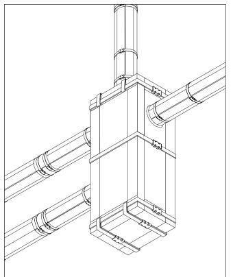
**Figure 4E:** Install steel banding around the box every 12 inches (30 cm) maximum and within 2 inches (5 cm) of each box edge and seam. It may be necessary to attach some banding to other bands, similar to the method shown on the bottom of the box assembly.
