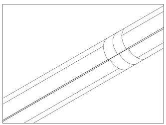
**Figure 2C:** Apply  $3M^{TM}$  425 Sealing Tape to all exposed E-Mat seams and edges.
