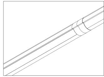
Figure 1B: Apply  $3M^{TM}$  425 Sealing Tape to all exposed E-Mat seams and edges.
