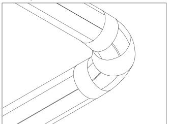
Figure 3D: Apply  $3M^{TM}$  425 Sealing Tape over all exposed seams and caulk.
