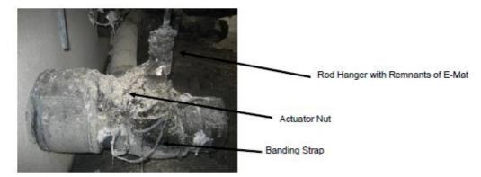
Figure 4-8 Specimen A Following Hose Stream Test
