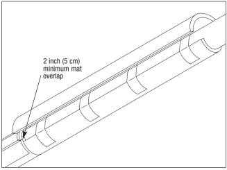
**Figure 1A:** Install first layer of 3M<sup>™</sup> Interam<sup>™</sup> Systems E-Mat tightly abutted to adjacent mat. Use 3M<sup>™</sup> 898 Filament Tape to secure mat to conduit. Mat must overlap 2 inches (5 cm) minimum onto itself.
