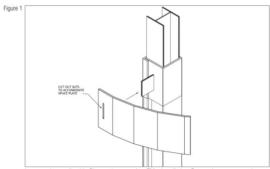
2 - Implement wrapping procedure outlined in Chapter 1 to complete EMat installation. Repeat the same procedure for all subsequent layers to achieve desired protection as per listing/design. 3M approved caulking to be applied around the penetrating item to provide an environmental seal to the EMat. This is to be completed after each layer of applied EMat.
