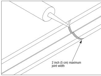
**Figure 2B:** Apply  $3M^{TM}$  Fire Barrier Sealant CP 25WB+ full depth to entire circumference of the butt joint between the mat wraps.
