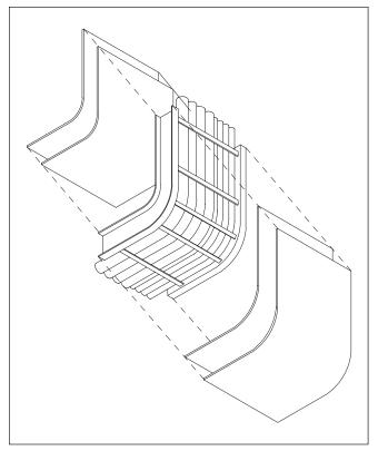
**Figure 5A:** Cut two 3M<sup>™</sup> Interam<sup>™</sup> Systems E-Mat inner and outer pieces (as shown) to the same width as the cable tray. Secure mat pieces using 3M<sup>™</sup> 898 Filament Tape.
