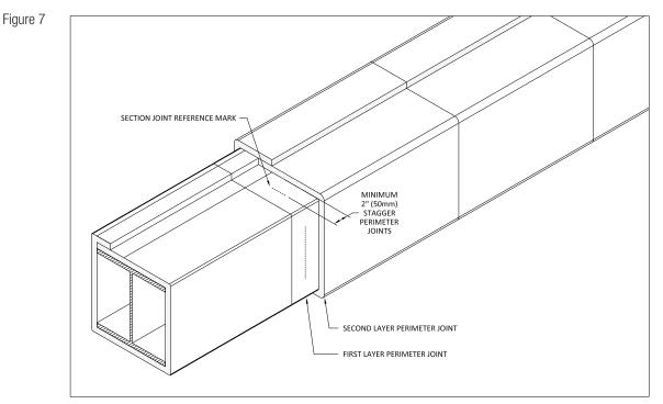
7 - Stagger all subsequent perimeter joints 2 inches from the previous layers' joint. Subsequent layers should be
