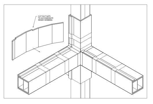
5 - Repeat steps 1 through 4 for all subsequent layers as per listing/design. The final layer where the EMat interfaces between the bottom and the top beams should be caulked by approved 3M caulking to prevent moisture from penetrating the joint.
