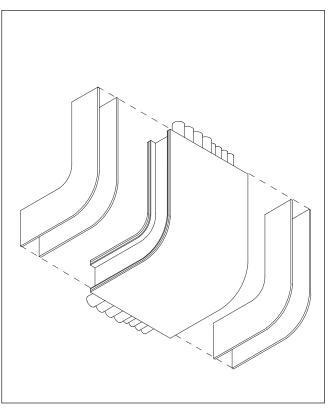
**Figure 5B:** Cut two E-Mat pieces for each side to fit over the cable tray sides and to cover edges of inner and outer E-Mat pieces already installed. Secure mat using  $3M^{TM}$  898 Filament Tape.
