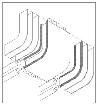
**Figure 6B:** Cut three pieces of E-Mat for each side of the cable tray. Cut the E-Mat pieces large enough to fit over the cable tray sides and cover edges of inner and outer wrap pieces already installed. Before installing side pieces, apply 3M<sup>™</sup> Fire Barrier Sealant CP 25WB+ to inner and outer E-Mat edges as shown. Install sides pieces and secure using 3M<sup>™</sup> 898 Filament Tape.
