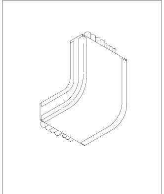
Figure 5F: Apply 3M<sup>™</sup> 425 Sealing Tape to all E-Mat seams.
