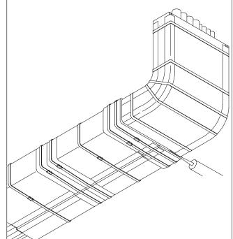
**Figure 7H:** Apply 3M<sup>™</sup> Fire Barrier Sealant CP 25WB+ to fill any gaps between the collar and the E-Mat sections underneath it. Apply steel banding within 2 inches (5 cm) of each collar edge, and at 12 inches (30 cm) maximum throughout the system.
