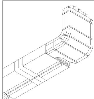
Figure 7F: Apply 3M<sup>™</sup> 425 Sealing Tape over all mat edges and seams.
