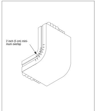
Figure 5D: Apply top and bottom E-Mat pieces as shown and secure using  $3M^{\text{TM}}$  898 Filament Tape.
