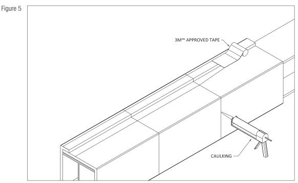
5 - The butt seam where the two pieces meet (perimeter joint) is to be covered with 3M approved tape. Tape and then mark the location of the joints on the tape using a soft tipped marker to establish a reference point. Smooth the tape with a hard roller or straight edge applying enough pressure to ensure adequate adhesion of the tape to the EMat and to remove any air gaps (Figure 6).
