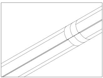
Figure 1E: Apply sealing tape over all exposed E-Mat seams and edges on the final layer.
