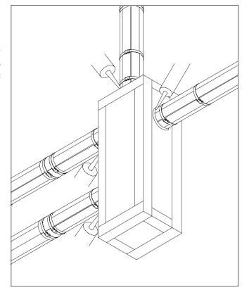
**Figure 4D:** Apply  $3M^{TM}$  425 Sealing Tape over all exposed mat seams and caulked edges. Apply  $3M^{TM}$  Fire Barrier Sealant CP 25WB+ around interface between wrapped conduit and box as shown.
