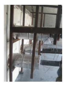
Figure 4-7 Side View of Unexposed Side Following Hose Stream Test
