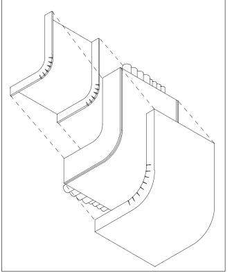
**Figure 5C:** Cut additional inner and outer E-Mat pieces so that they overlap onto the side pieces by at least 2 inches. (5 cm). Cut "slits" into the radius area of the overlap.
