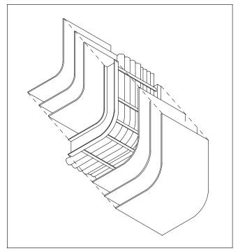
**Figure 6A:** Cut three  $3M^{TM}$  Interam<sup>TM</sup> Systems E-Mat inner and outer pieces (as shown) to the same width as the cable tray. Secure mat using  $3M^{TM}$  898 Filament Tape.
