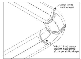
**Figure 3B:** Install narrow sections of mat in continuous manner as shown. These sections should touch on the inner radius. Each section should have a final layer overlap of at least 6 inches (15 cm). Secure each section into place using 3M<sup>™</sup> 898 Filament Tape.
