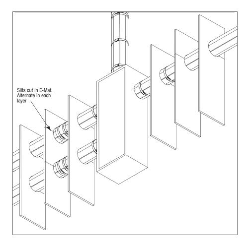
Figure 4A: Install 3M<sup>™</sup> Interam<sup>™</sup> Systems E-Mat on all conduit attached to circuit box first. See Figures 1, 2 and 3 for information on wrapping conduit. E-Mat on conduit should tightly abutt box.
