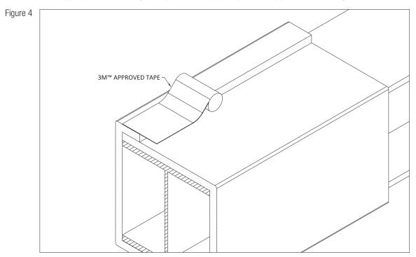
4 - For the next section of wrap, repeat steps 1 through 3. The next section of Emat should be tightly abutted to the first section eliminating all gaps when possible. If a gap of more than 1/8 inch (3 mm) remains in the perimeter joint between sections of EMat, the gap is to be filled to the full depth of the Emat with an approved 3M sealant (Figure 5).
