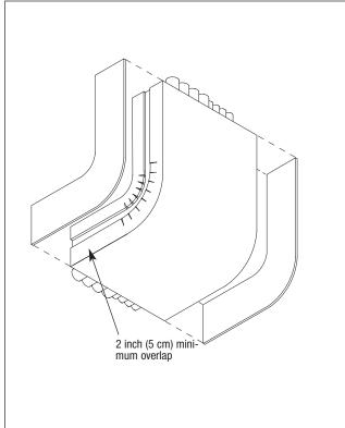
**Figure 5E:** Cut and install the third side layer of  $3M^{TM}$ Interam<sup>TM</sup> Systems E-Mat as shown. Secure mat using  $3M^{TM}$  898 Filament Tape.
