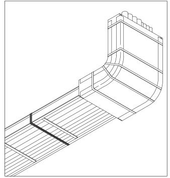
Figure 7A: Install 3M<sup>™</sup> Interam<sup>™</sup> Systems E-Mat to cable tray elbow sections following steps 5A to 5G or steps 6A to 6D.
