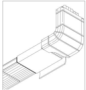
**Figure 7B:** Wrap first layer of E-Mat around the cable tray straight section. Complete the layer with a 2 inch (5 cm) minimum overlap. Secure mat using 3M<sup>™</sup> 898 Filament Tape.
