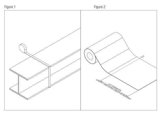
2 - Cut Endothermic Mat 5A-4 (EMat) to length using bladed edge. Align EMat to the steel with foil side facing outward (white side should be in contact with steel). Edge of EMat can be held in place by filament tape or by other worker. Wrap EMat around the steel then overlap itself by a minimum of 2 inches (50 mm) (Figure 3). Additional overlap is acceptable but not required. EMat should be tight to the steel, free of slack.
