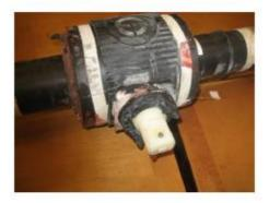
Figure 4-10 Close-up of Valve Operator and Remnants of Actuator Nut
