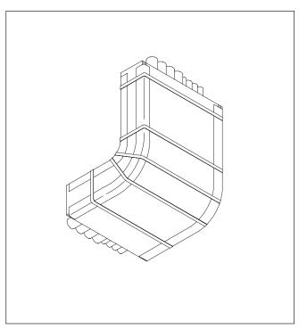
**Figure 6D:** Install steel banding around the cable tray every 12 inches (30 cm) maximum and within 2 inches (5 cm) of each cable tray end. See Figures 7A to 7H for details regarding a transition of the cable tray elbow to a cable tray straight section.
