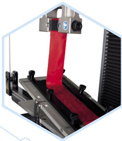
Figure 7: Experimental set up for adhesion to steel measurement at an adjustable peel angle.
