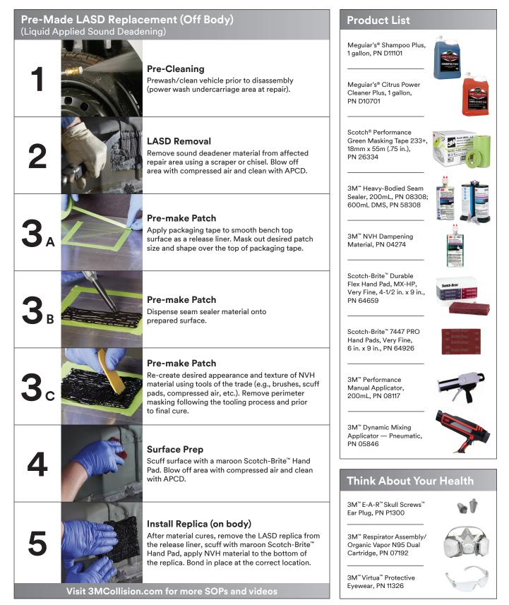
Note: Pre-made LASD replacement patches are typically created off body for panels with complex surfaces.
