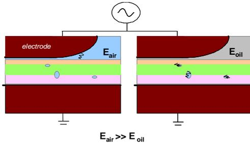
The ability to detect enclosed air in an oil environment was demonstrated using a microstructured film laminated to a pressure sensitive adhesive, with increasing amounts of pressure (Figure 7). This had the effect of creating air bubbles of different sizes, which were measured microscopically.
