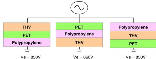
**Surface effects.** Out of the four categories of partial discharge listed earlier, both surface and internal discharges are of concern with regards to potential for erosion of insulating material, and subsequent deterioration of its insulating properties.<sup>8</sup> It is well known that an air corona can impact the surface of a polymer<sup>9,10,11</sup>, as a result of secondary reactions following the ionization of air:
