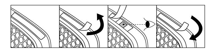
The ESLI is covered by a repositionable tab to help protect it from overspray and debris. Pull back the tab to view the ESLI. Ensure that the ESLI is intact and uniform in appearance. The indicator bar may be green on a red background or red on a green background, depending on the viewing angle. Rotate the cartridge slightly while looking at the indicator. (Refer to the User Instructions for more information.)
