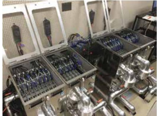
The Suiren requires only 68 square feet of space. Because the system is designed with immersion cooling using 3M Fluorinert Electronic Liquid, the servers do not require fans to blow air, eliminating additional fan noise.
